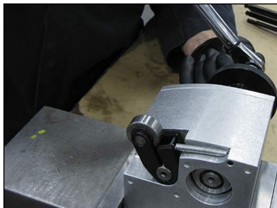
FIGURE 5-4. ADJUSTING CAM ARM SCREW TO CORRECT TORQUE VALUE
