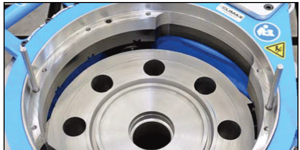
FIGURE 3-18. 5/16" RODS FOR MANUALLY ROTATING THE RDU BEARING (FF1200 SHOWN)
