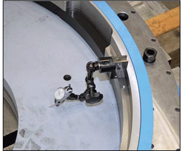
FIGURE 3-17. LEVEL THE RDU (FF3600 SHOWN)
