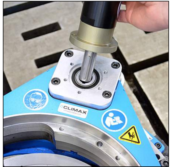
FIGURE 3-24. ALIGN THE AIR MOTOR (FF1200 SHOWN)
