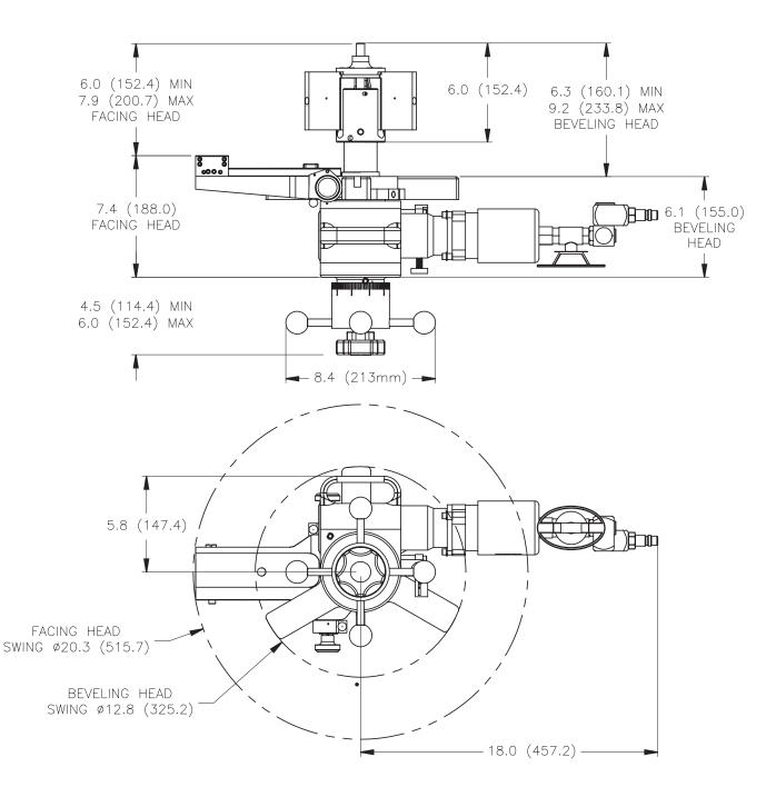
Note: Facing and Beveling heads shown for dimensional reference only. They can not be mounted simultaneously.
